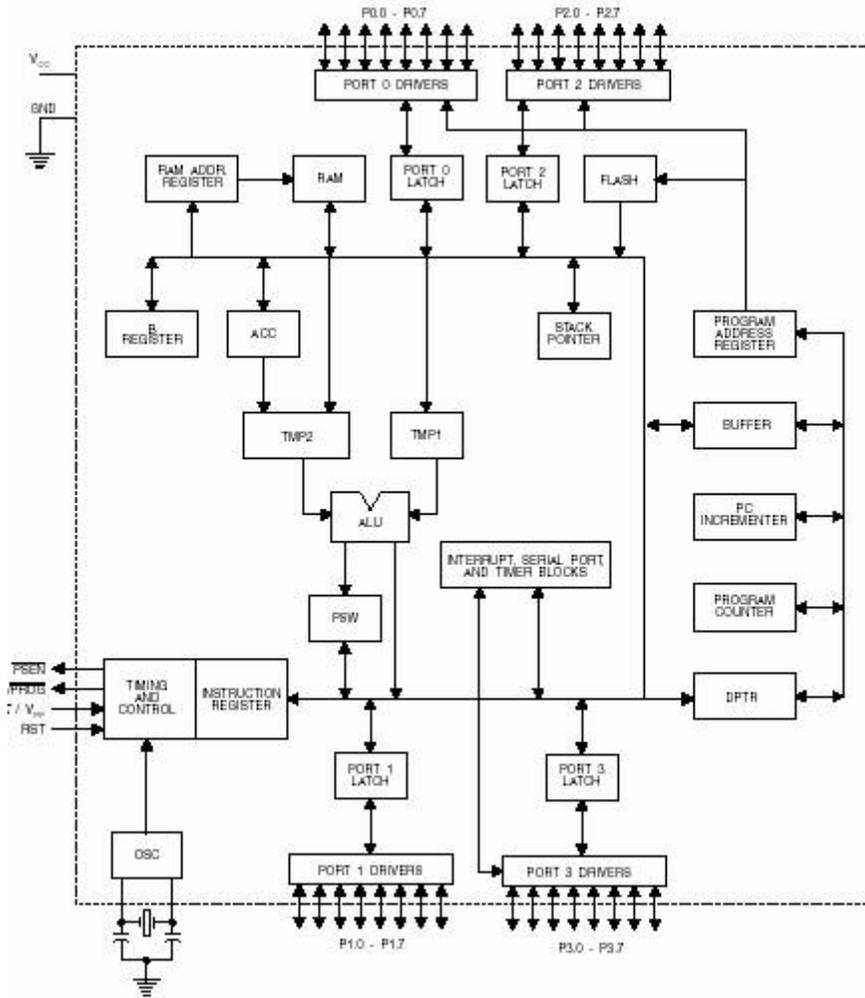
Gambar Diagram Blok MCS-51 Sumber : Atmel, 1997 : 4 – 30
